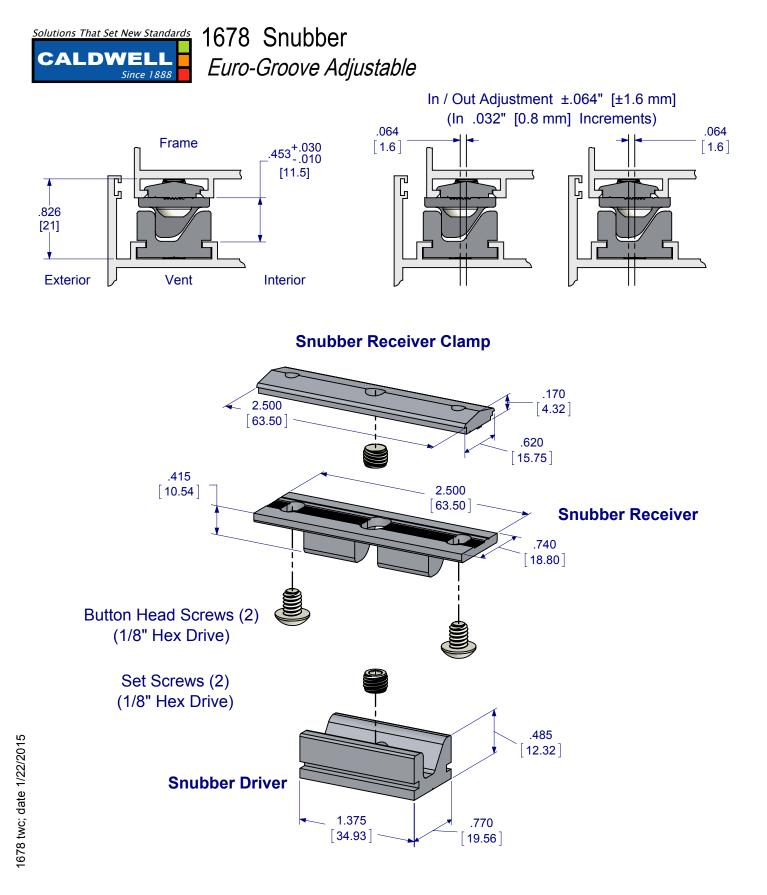
Positive and negative pressure containment. Adjustable ±0.064" [±1.6 mm] . #1678 Snubber includes driver, receiver, clamp, set screws and button head screws. Material: 6000 series aluminum with black coating.
