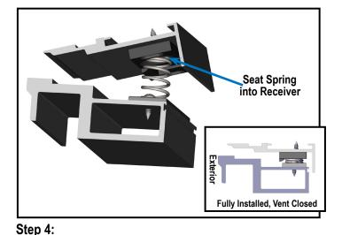
As vent is brought closed, ensure that the spring seats into the Snubber Receiver by pushing it towards the exterior.
