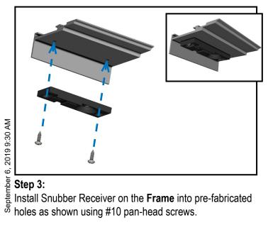
Install Snubber Receiver on the Frame into pre-fabricated
