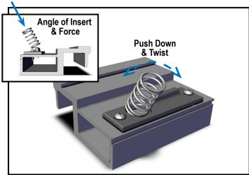
Step 2: With the closed end of the spring facing towards you angle the spring down, twist back and forth, and apply force to the back of the spring until the spring engages and snaps under the Spring Retention Feature on the Snubber Driver. Then rotate the spring counterclockwise until tight against vent.
