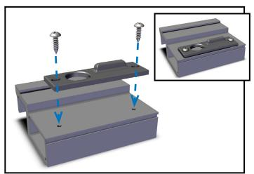
Step 1: Install Snubber Driver on the **Vent** into pre-fabricated holes from CO\_20J0069 as shown, using #10 pan-head screws.
