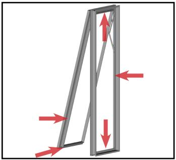
**Step 1:**Open the Vent. Clean any dirt, debris or foreign matter from the Vent and Frame surfaces as needed.
