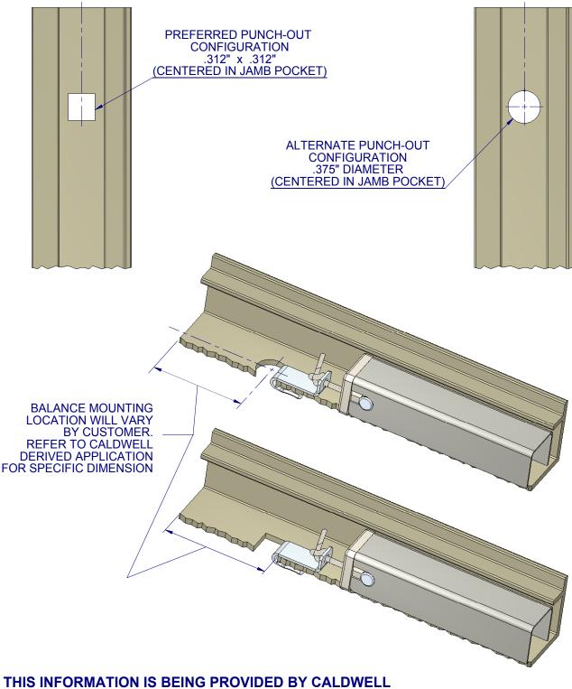
THIS INFORMATION IS BEING PROVIDED BY CALDWELL TO PROVIDE OPTIMAL INSTALLATION CONDITIONS FOR HOOK MOUNT PRODIGY™. OTHER SIZES HAVE BEEN FOUND TO PROVIDE ACCEPTABLE RESULTS.
